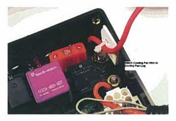
NOTE: Do not use power tools to tighten eyelet retaining nut, damage to the circuit board may occur if overtightened!
