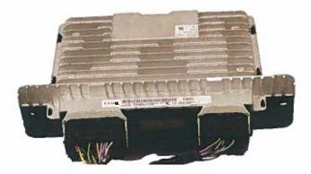
NOTE: Due to the fuel system requirement described above, installation of this PCM in ANY Production Mustang vehicle will result in a no-start condition!
