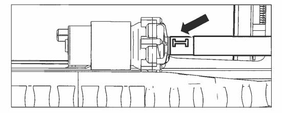
7. Route the remainder of the Intercooler Pump Wiring Harness and secure. Connect the wiring harness to the pump and secure the harness to the bracket using the holes in the intercooler pump mounting bracket.
