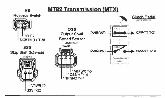
NOTE: All connector views are looking into the connector's face with the wires flowing away from the viewer.
