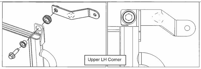
4. Repeat step 3 for each of the remaining LTR Brackets. 13108K243 will go to the upper RH corner, 13108K244 to the lower LH corner and 13108K245 to the lower RH corner of the LTR. These can be found in Hardware Kit E (13116066FRTHKE).
