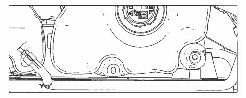
2. Install (1) M6 J-Clip (N623332) from Hardware Kit E onto the fan shroud. Reinstall the fan shroud and bolts and torque to 10 Nm. Reinstall the intercooler degas bottle using (2) M6 x 1.0 x 22 mm bolts (R18020057) and torque to 10 Nm.
