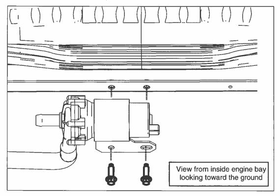
5. Connect the Intercooler Pump to LTR hose to LTR inlet port using (1) ¾" constant tension clamp. Orient the clamp so the "I" on the hose is in the center of the clamp tangs.
